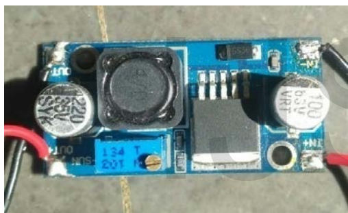
Fig.5: LM2576 Buck Converter circuit
